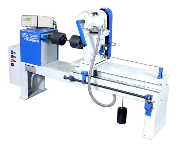
Suitable for Torsion and Twist tests on various meta rods and flats.
